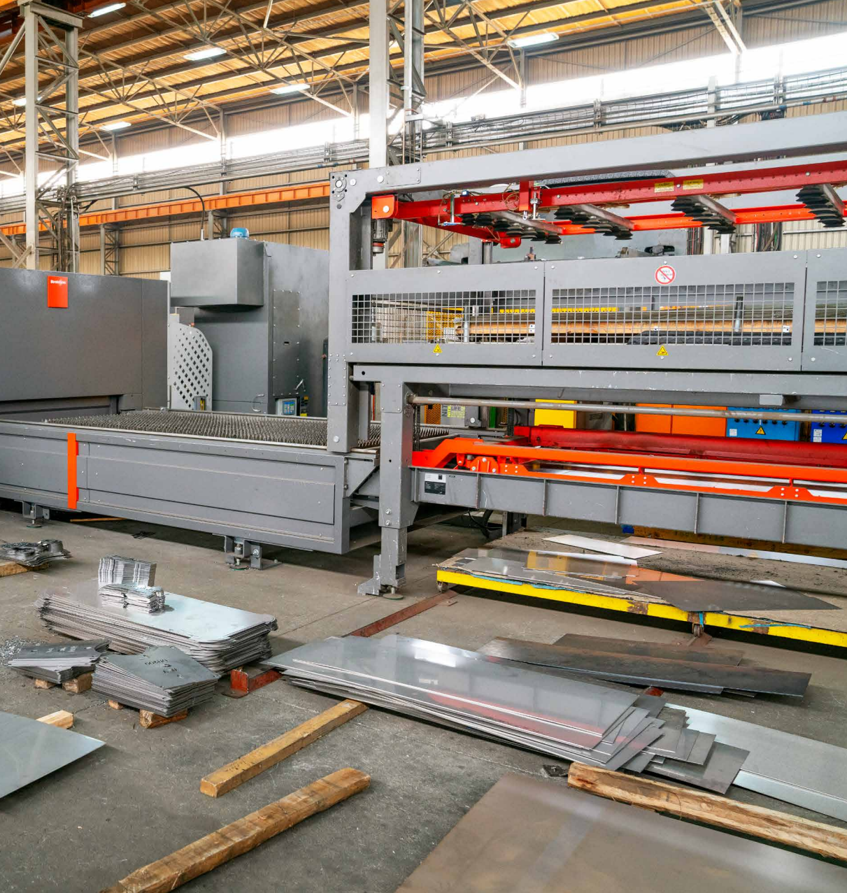
The BySmart 3015 3kW fiber laser with the ByTrans Cross automation solution helps speed up the vast production volumes.
